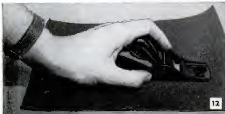
Bottom of a hand plane is easily polished by rubbing on a piece of emery cloth placed on flat surface. Use fine abrasive
